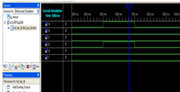
Fig 17 : Results for asynchronous reset circuit
